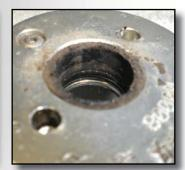
Abused shafts and not cleaning off excess dirt from the shaft and seals can over time eat away at the seals and change the seals rubricity
